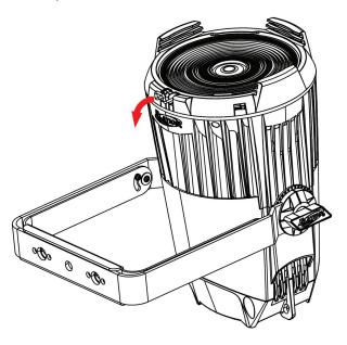
2. Slide the barn door into place in one of the vacant accessory slots on the front of the fixture.
